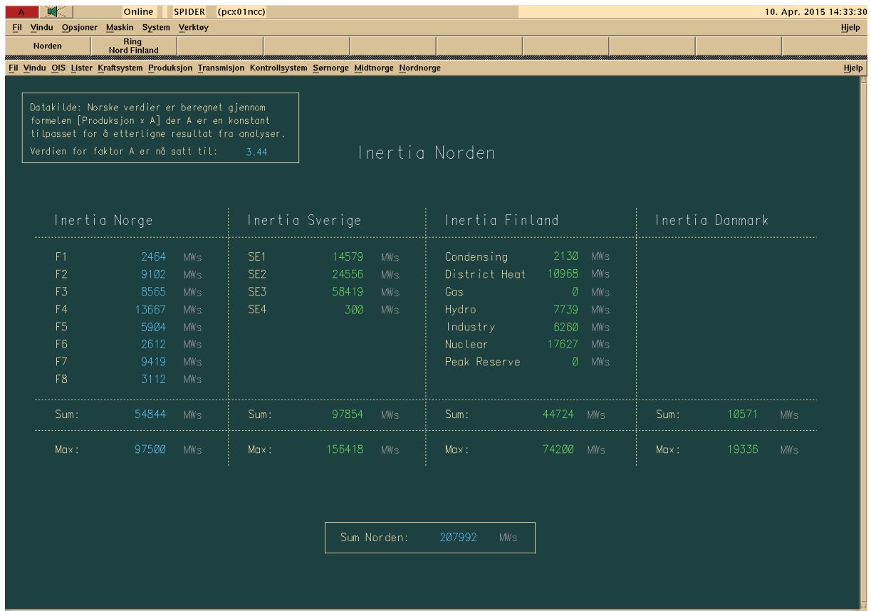
FIGURE 4.4: STATNETT SCADA VIEW FOR PRESENT SOLUTION.
