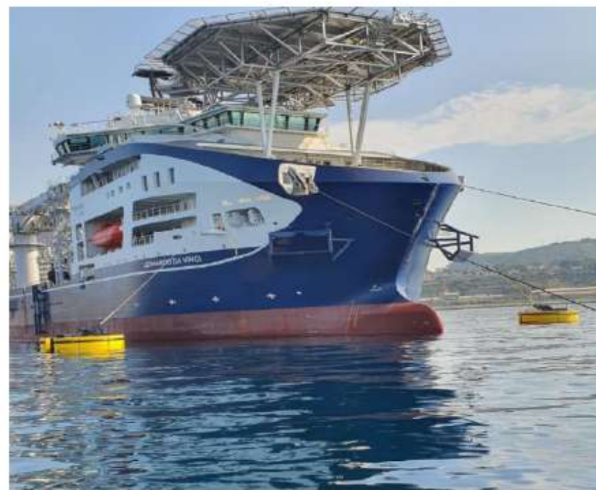
C2 HVDC Cable Load – LDV - Port & Starboard FWD moorings with two Bow anchors deployed.
