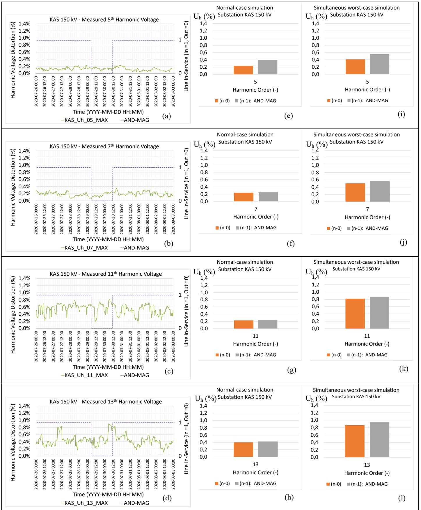
Fig. 8. Harmonic voltage distortion in the substation KAS as response to the AND-MAG line switching event: (a), (b), (c), (d) – measured, (e), (f), (g), (h) – simulated normal case, and (i), (j), (k), (l) – simulated simultaneous worst case. The measurements and simulations are shown as the maximum magnitudes of the three phases of the harmonic voltage. The arrows mark steps of the harmonic voltage magnitudes.
