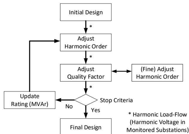
Fig. 13. Process of the harmonic filter design for the meshed transmission grid.
