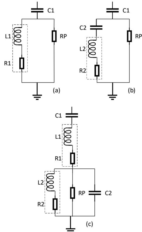
Fig. 12. Harmonic filter types: (a) – high-pass 2<sup>nd</sup> order filter (b) – C-type filter, and (c) – double-tuned filter.
