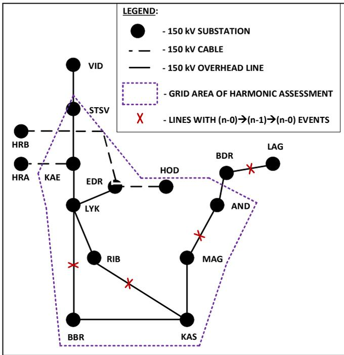
Fig. 4. Operation conditions with (n-1) events in the 150 kV grid, the 2020/2021 grid development stage. The events are registered one at a time.
