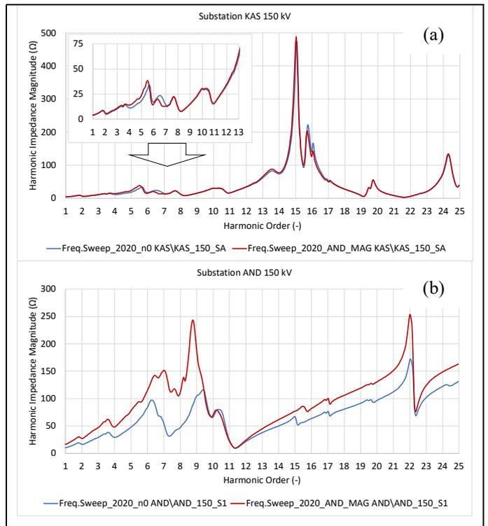
Fig. 16. Harmonic impedance magnitude for the present 2020/2021 grid in the substations: (a) – KAS, (b) - AND. Blue curves – (n-0) and red curves – (n-1) for the AND-MAG 150 kV line out-of-service.
