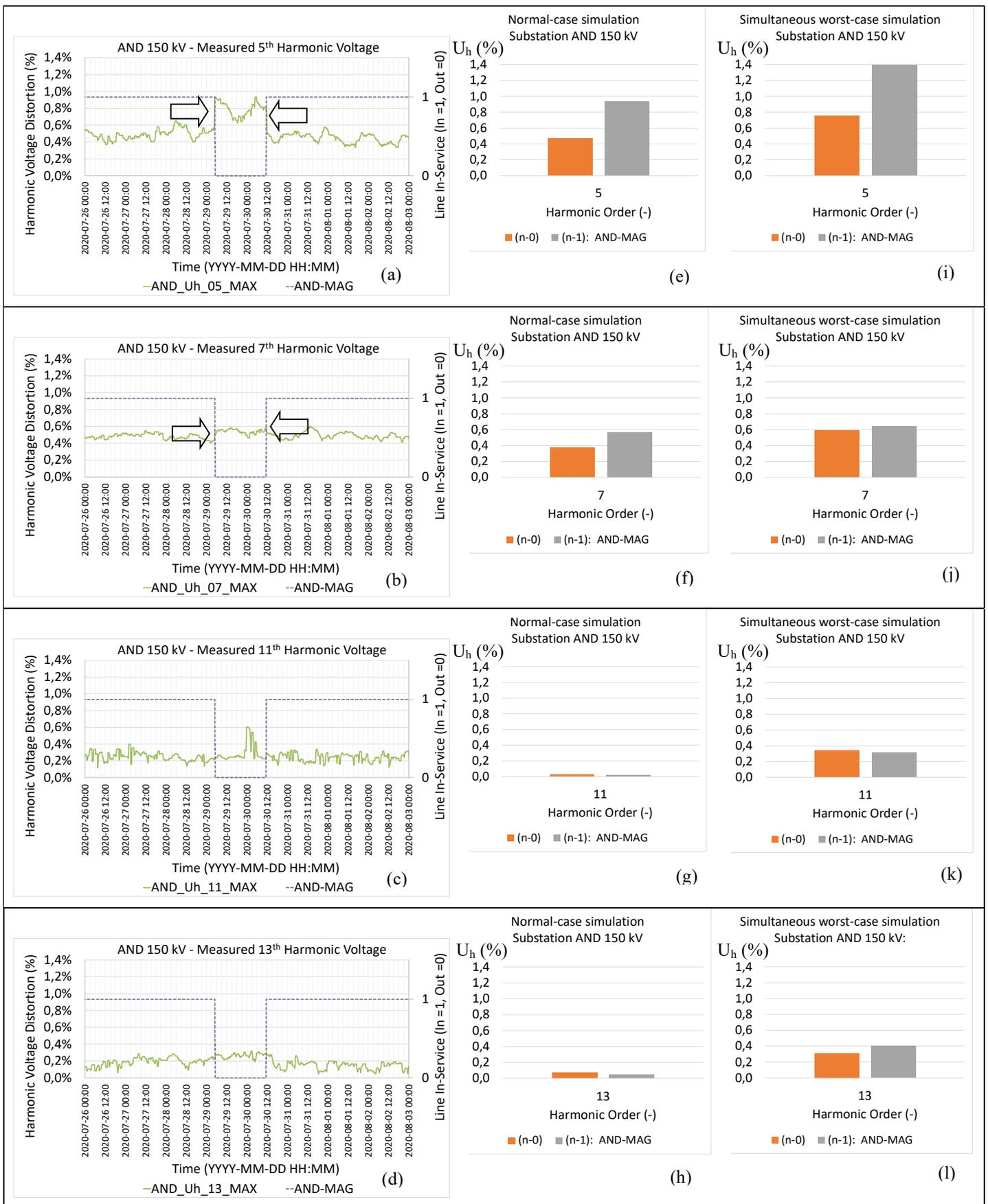
Fig. 7. Harmonic voltage distortion in the substation AND as response to the AND-MAG line switching event: (a), (b), (c), (d) – measured, (e), (f), (g), (h) – simulated normal case, and (i), (j), (k), (l) – simulated simultaneous worst case. The measurements and simulations are shown as the maximum magnitudes of the three phases of the harmonic voltage. The arrows mark steps of the harmonic voltage magnitudes.
