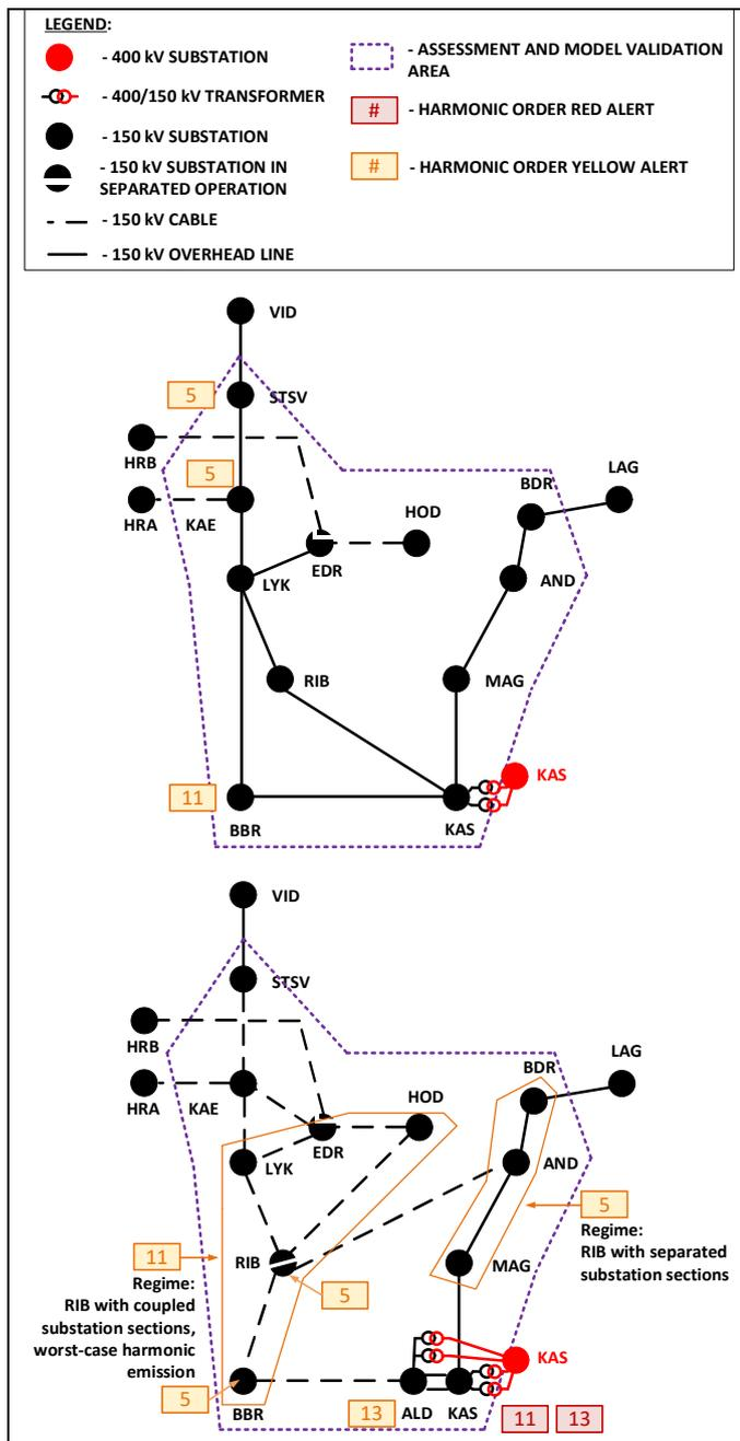
Fig. 11. Harmonic voltage distortion in the Kassø-Lykkegård 150 kV grid area with indication of yellow and red alerts: (a) – present 2020/2021 grid and (b) – reconstructed grid.
