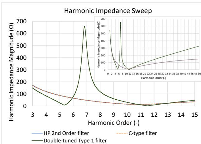
Fig. 14. Harmonic impedance sweeps of the three assessed filter types.
