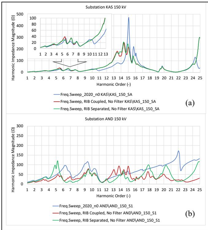
Fig. 17. Harmonic impedance magnitude in the substations: (a) – KAS, (b) – AND. Blue curves – the present 2020/2021 grid, red curves and green curves – the reconstructed grid with coupled and separated operation of RIB, respectively.
