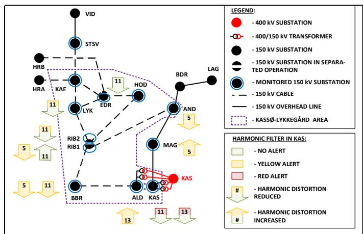
Fig. 15. Results of the combined performance and detuning study of the high-pass 2<sup>nd</sup> order filter in the 150 kV substation KAS.
