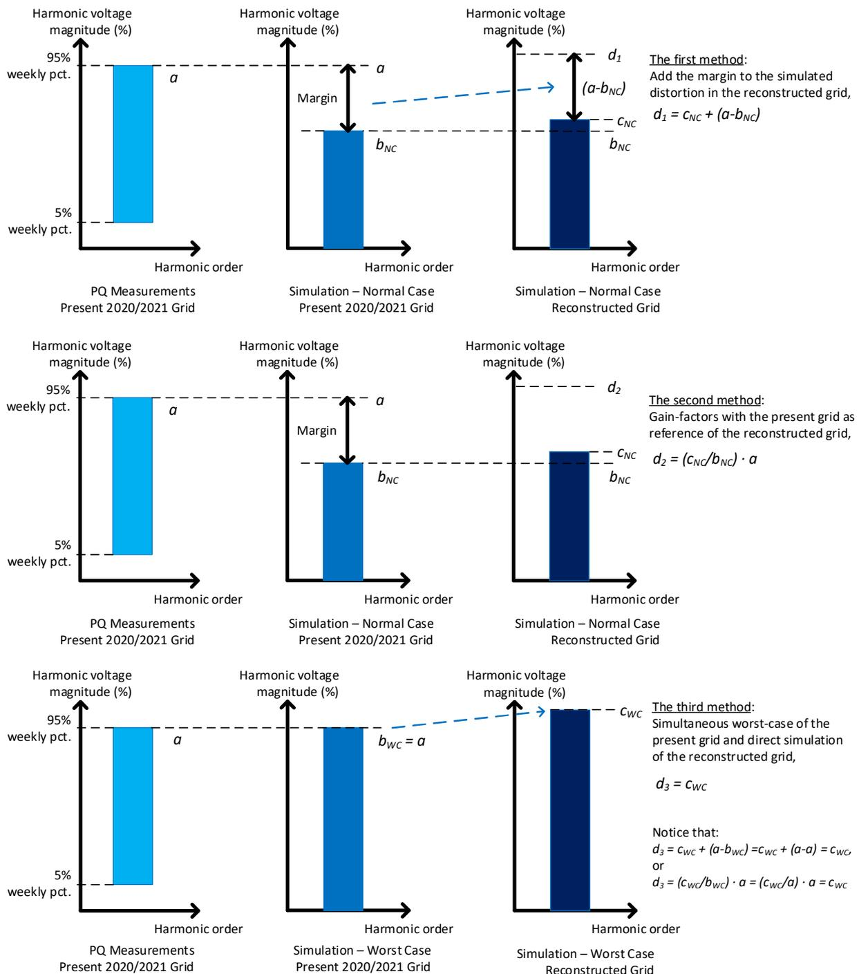
Fig. 9. Illustrations of the three methods for determining the simulated harmonic voltage distortion in the reconstructed grid: (a) – the first arithmetical method, (b) – the second gain-factor method, (c) – the third direct method.
