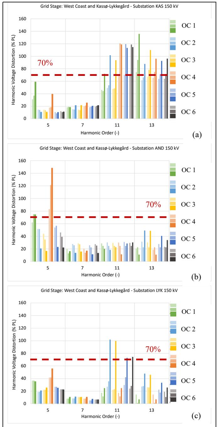
Fig. 10. Harmonic voltage magnitudes in the substations (a) – KAS, (b) – AND, and (c) – LYK, of the 150 kV reconstructed grid. Depicted operation conditions:
