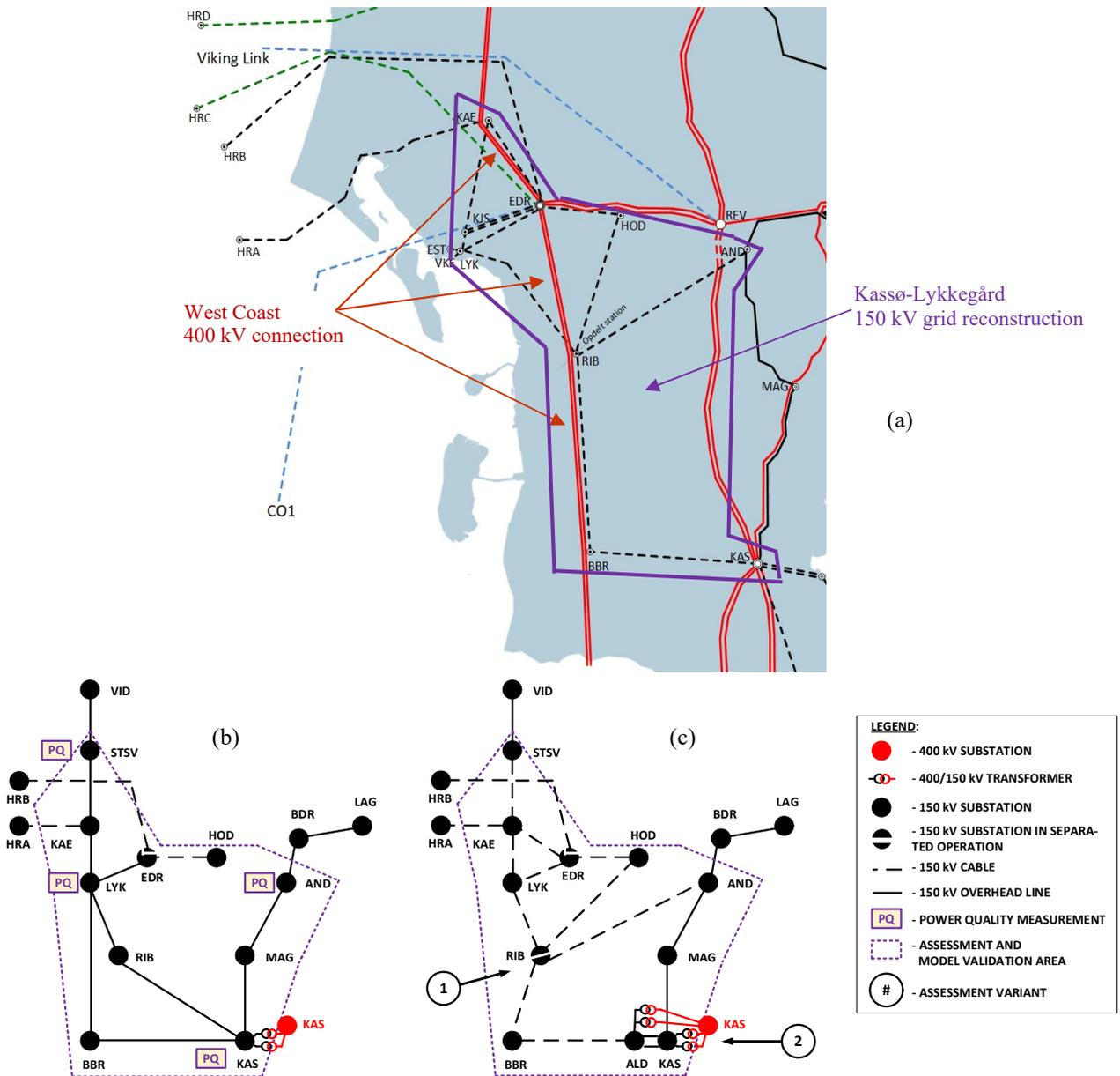
Fig. 2. The Kassø-Lykkegård grid reconstruction area in the transmission system of Western Denmark: (a) – reconstructed grid of Southwestern Jutland with solid magenta line marking the project area, (b) – the 2020/2021 grid development stage and (c) – the 2023 grid development stage after completed grid reconstruction with the UGC. The stipled magenta line marks the harmonic assessment area. PQ marks the 150 kV substations with the PQ measurements available at the time of the assessment.
