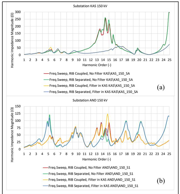
Fig. 18. Harmonic impedance magnitude for the reconstructed grid in the substations: (a) – KAS, (b) – AND. Red curves and green curves – no harmonic filter and with coupled and separated operation of RIB, respectively. Yellow curves and blue curves – harmonic filter in KAS and with coupled and separated operation of RIB, respectively.
