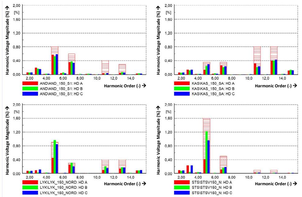
Fig. 5. Normal case. Comparison of the simulated harmonic voltage magnitudes to the maximum (measured) 95<sup>th</sup> weekly percentiles in the four 150 kV substations with available PQ measurements: AND, KAS, LYK, and STSV.
