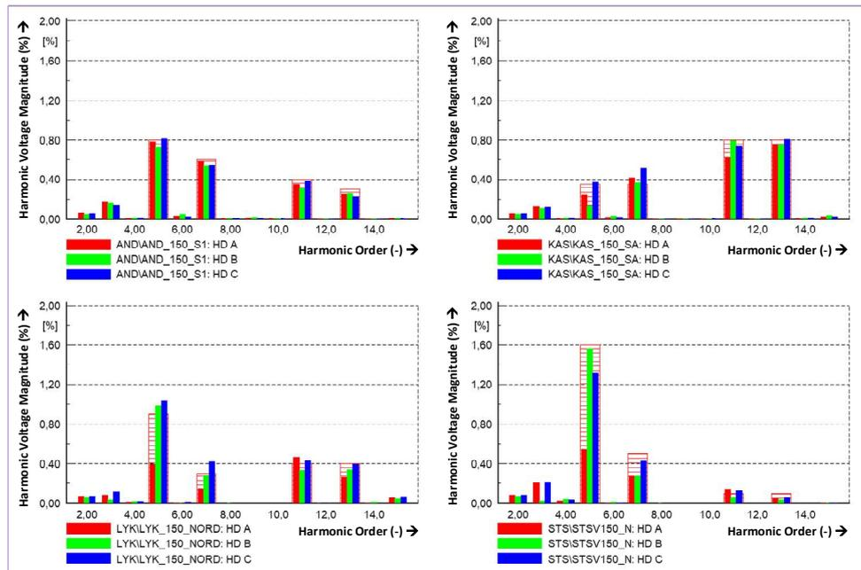
Fig. 6. Simultaneous worst case. Comparison of the simulated harmonic voltage magnitudes to the maximum (measured) 95<sup>th</sup> weekly percentiles in the four 150 kV substations with available PQ measurements: AND, KAS, LYK, and STSV.
