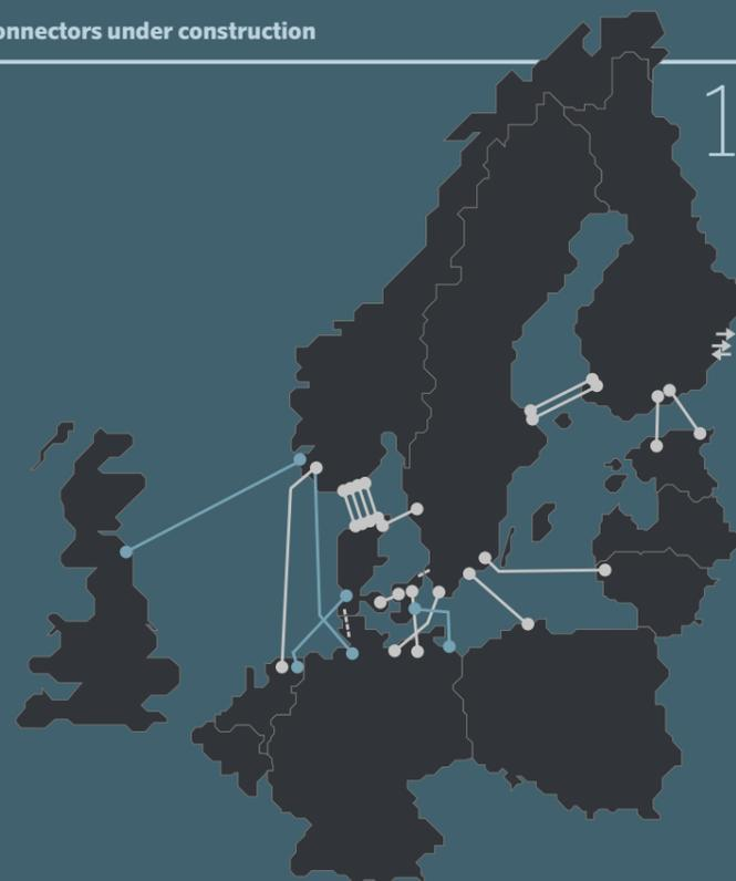
Figure 1 Overview of existing and planned HVDC interconnectors in the Nordic power system. Only those planned HVDC interconnectors with a final investment decision are included.
