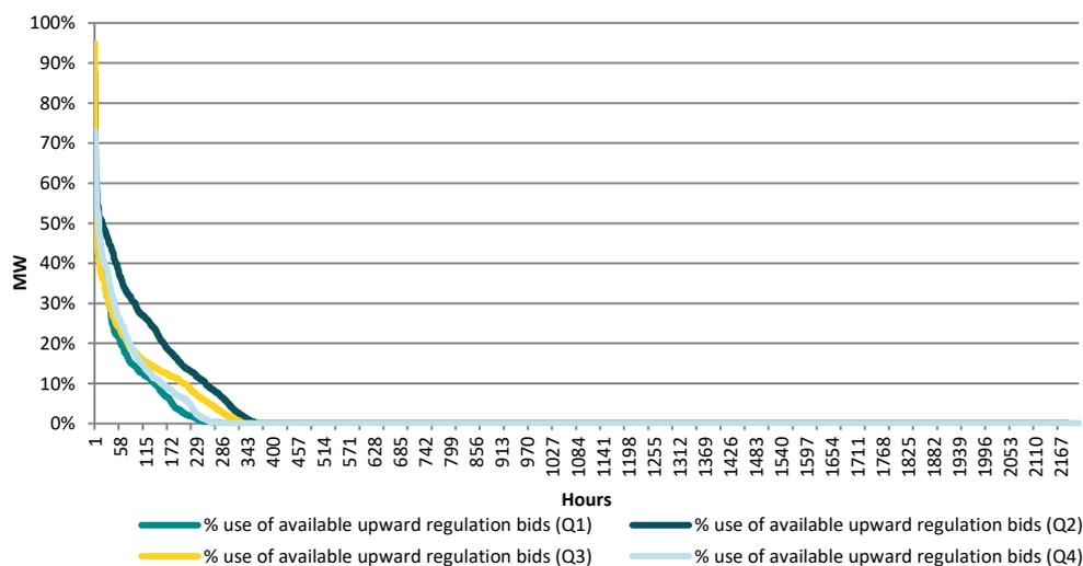
Figure 3: Duration curve of % use of offered upward regulation in DK1.
