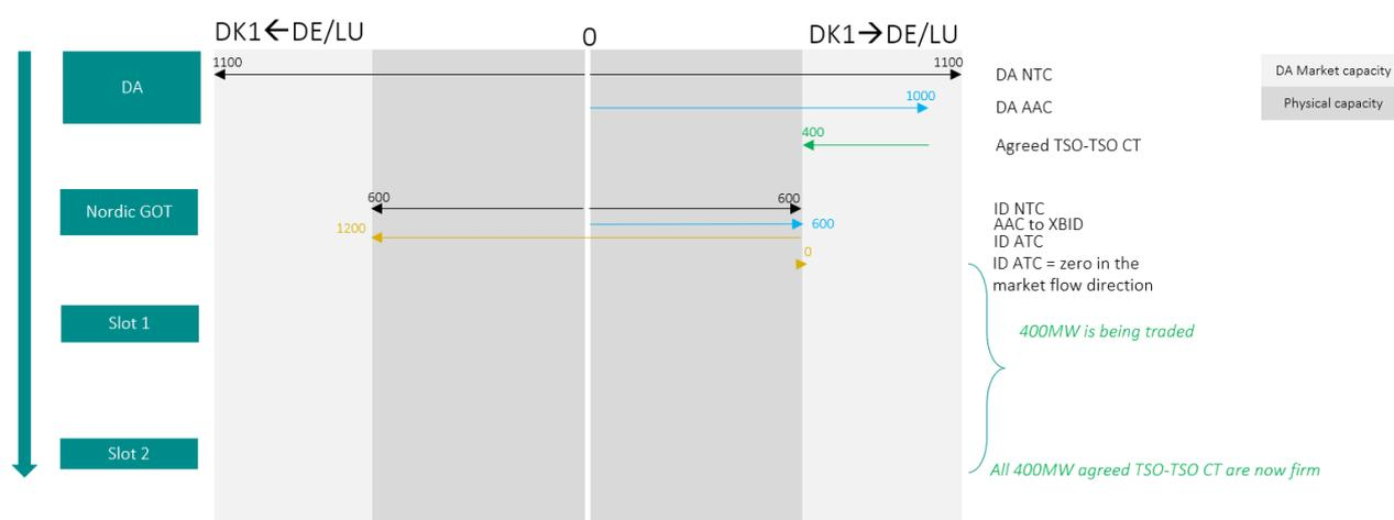
Figure 9:  $ATC_{ID}$  is 0 MW in the market flow direction after taking countertrade into account. The capacity in the opposite direction of the market flow is 1200 MW, as there is a physical flow in the market flow direction of 600 MW.
