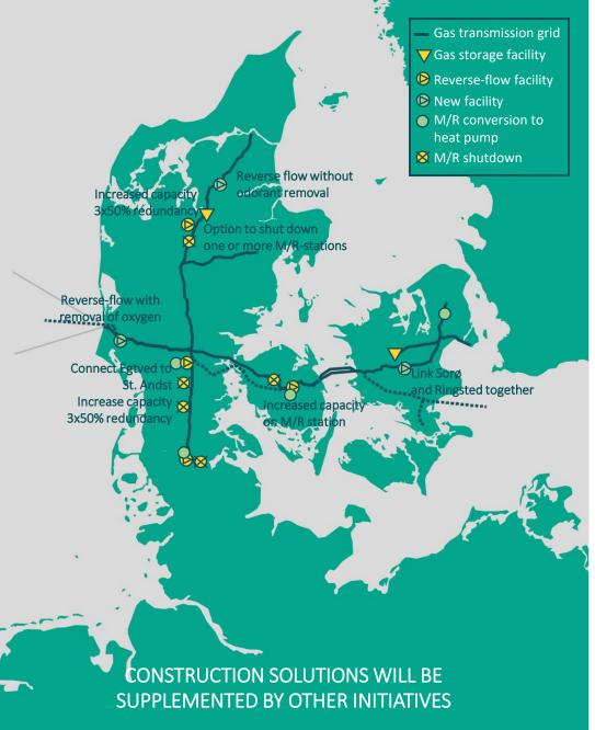
The map shows an overall package of possible changes to the gas transmission grid and is intended to illustrate how much work is required to convert the gas system to green supply.
