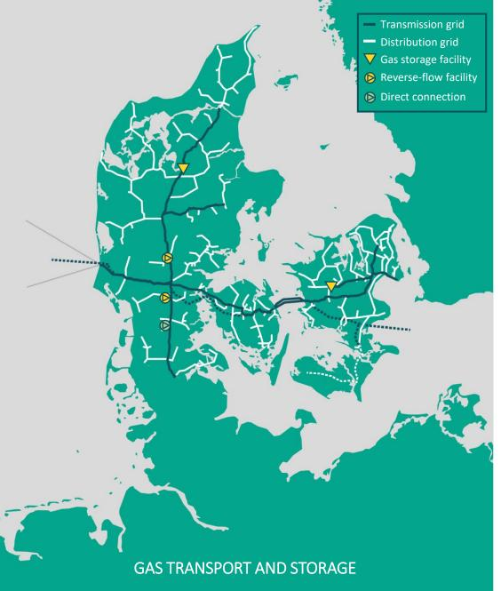
Danish gas consumers are supplied via the distribution grid which is the responsibility of Evida. The distribution grid is connected to the gas highway – the transmission grid – through Energinet's metering and regulator stations (M/R stations) throughout the country.
