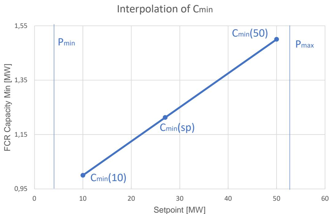
**Figure 33.** Second step of the linear interpolation to determine the minimal capacity for setpoints between the minimum and maximum tested setpoint.
