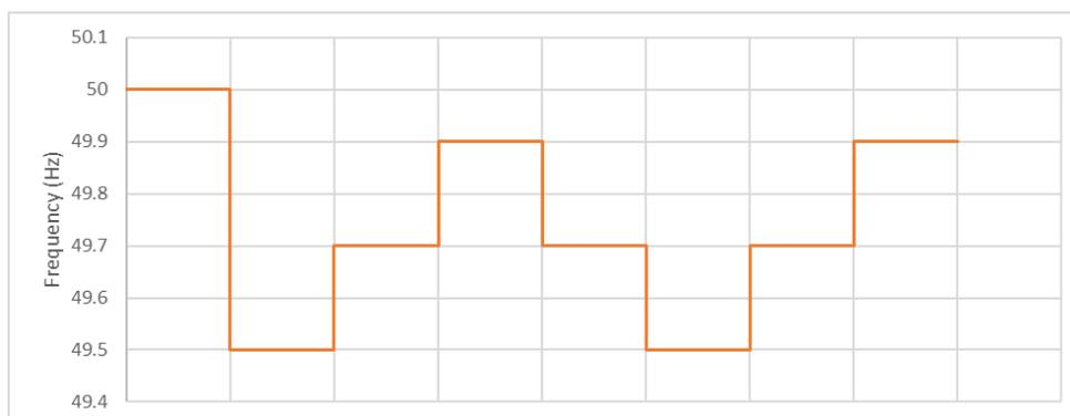
Figure 5. Input frequency signal for FCR-D Upwards step response tests
