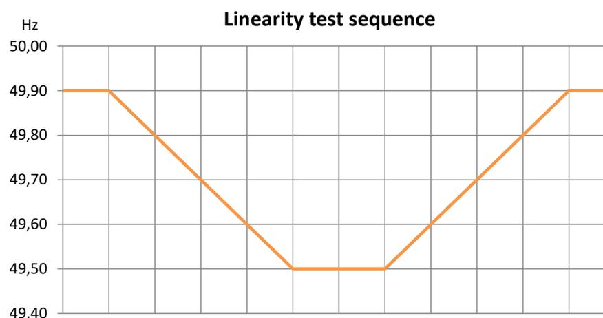
**Figure 12. FCR-D upwards linearity test sequence to be performed for each setpoint and parameter set.**
