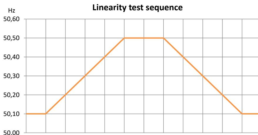
Figure 13. FCR-D. downwards linearity test sequence to be performed for each setpoint and parameter set.
