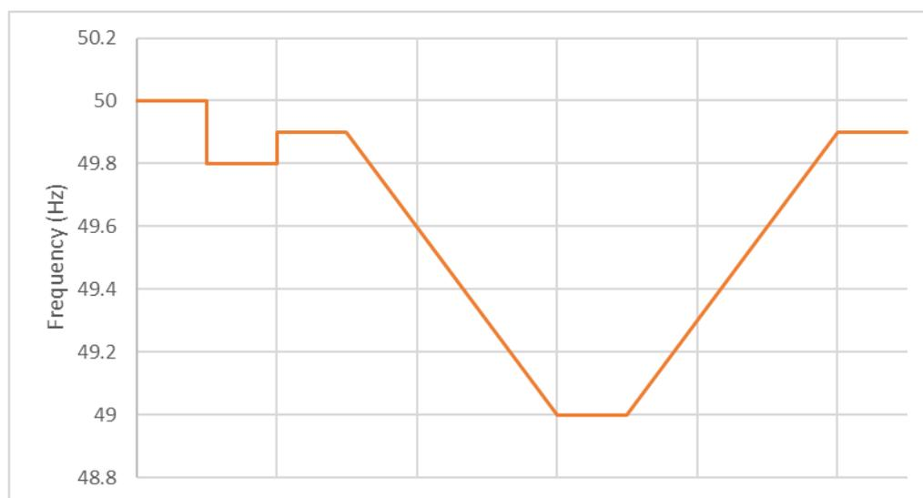
Figure 6. Input frequency signal for FCR-D Upwards ramp response tests
