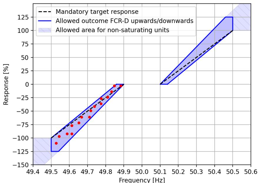
Figure 31. Example response (red dots) of stationary activation of FCR-D Upwards for a demand response FCR providing entity, compared to requirement for linearity (blue area).
