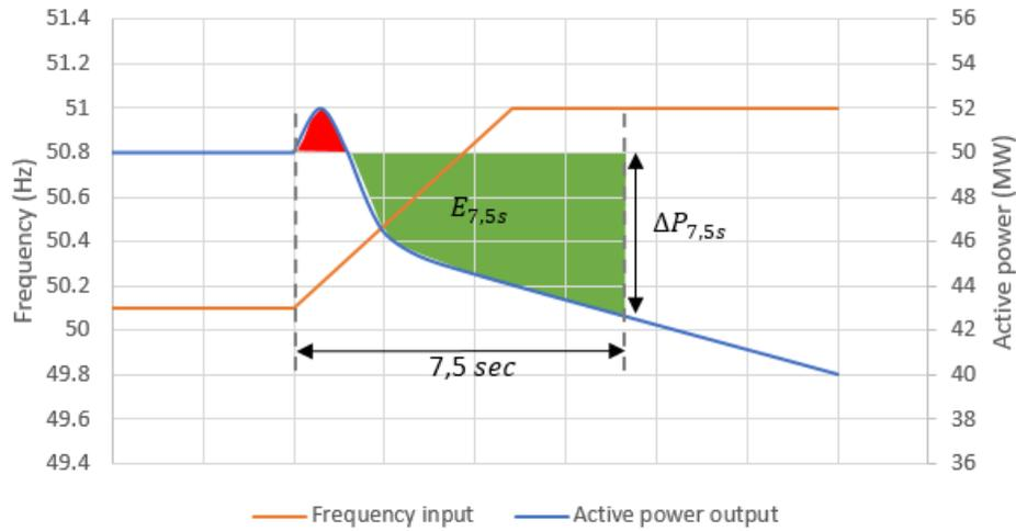
**Figure 28: Example response (blue) from input frequency (orange) according to ramp test sequence for evaluation of FCR-D downwards performance**
