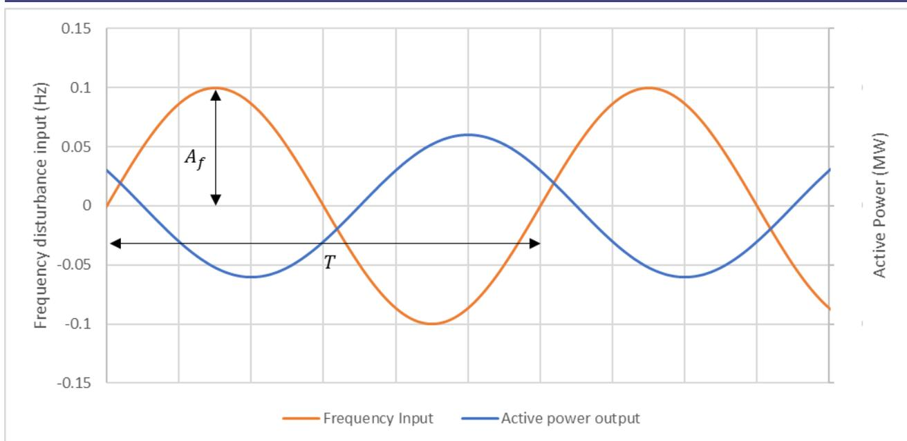
Figure 10. Input frequency signal for FCR-D sine tests
