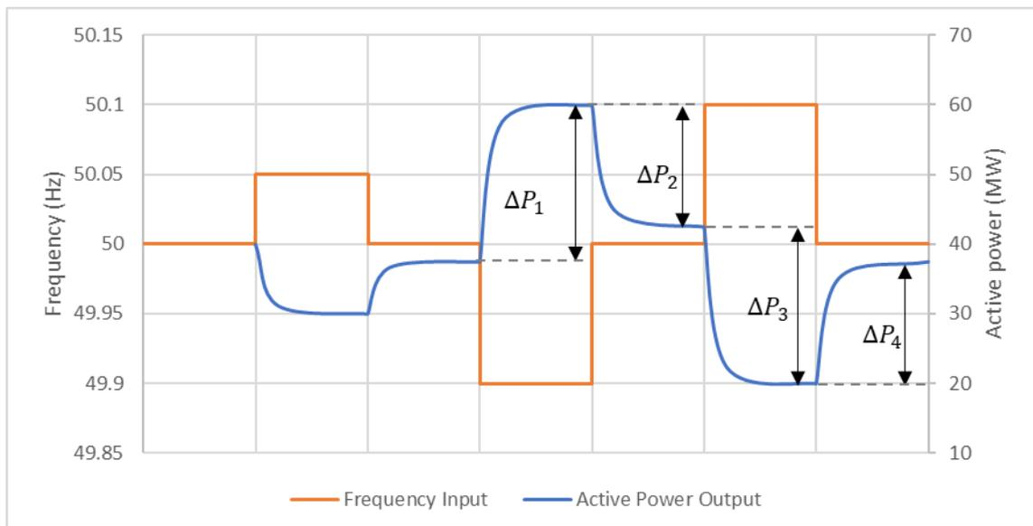
Figure 20. Example response (blue) from input frequency (orange) according to FCR-N step test
