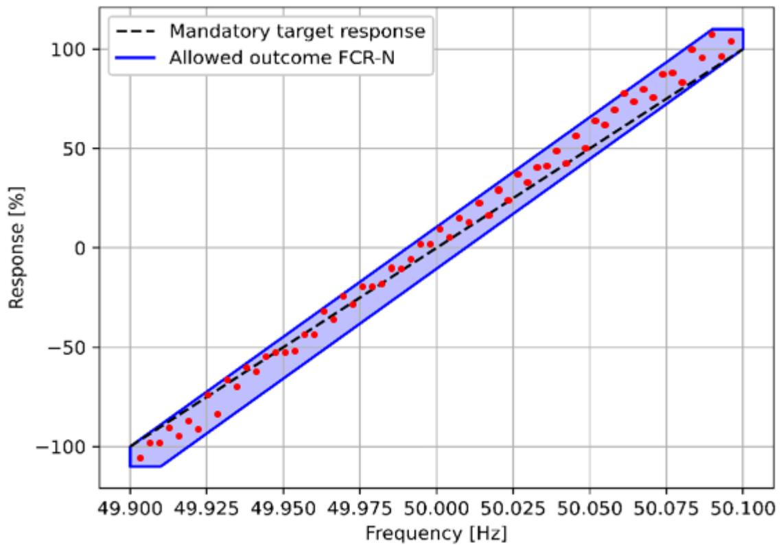
Figure 30. Example response (red dots) of stationary activation of FCR-N for a demand response FCR providing entity, compared to requirement for linearity (blue area).
