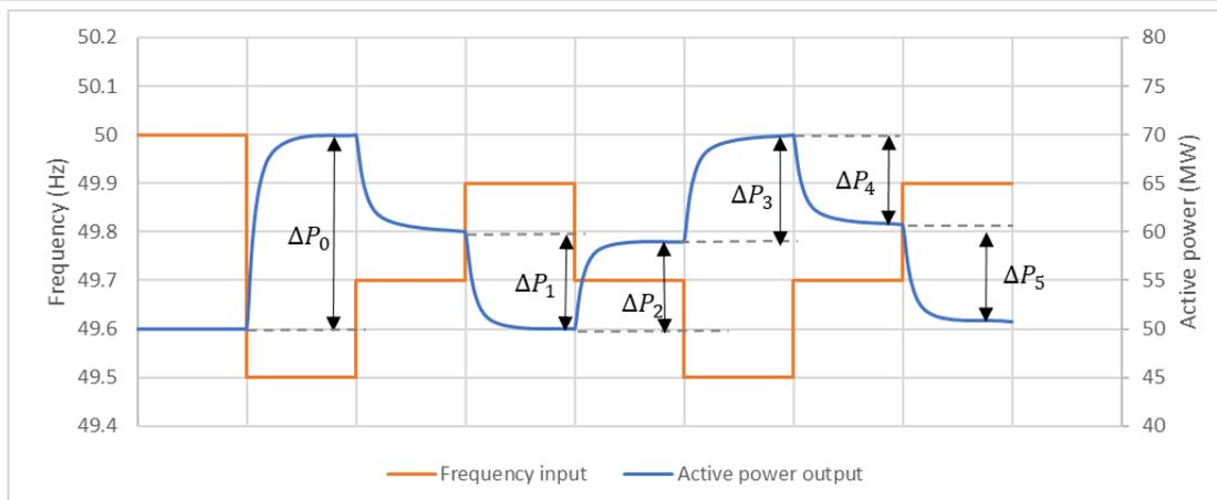
Figure 24. Example response (blue) from input frequency (orange) according to FCR-D Upwards step test
