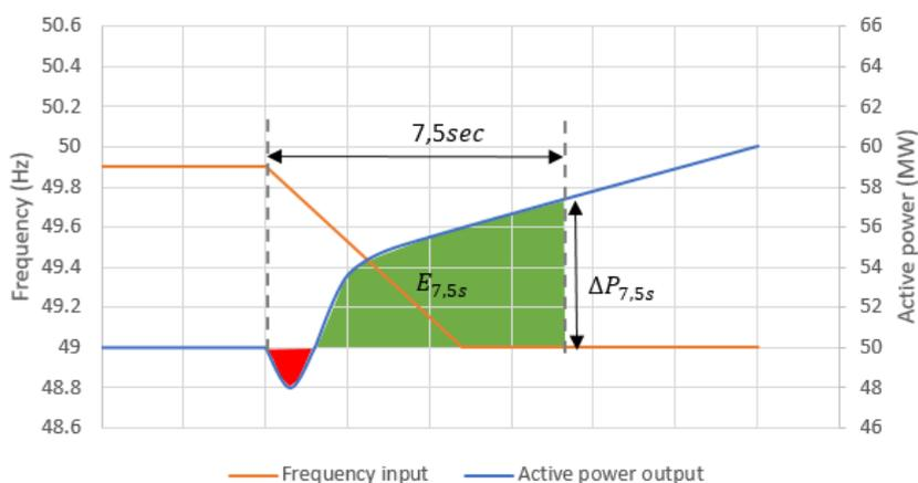
Figure 25: Example response (blue) from input frequency (orange) according to ramp test sequence for evaluation of FCR-D upwards performance
