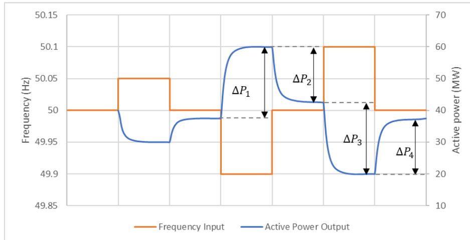
Figure 14. Example response (blue) from input frequency (orange) according to FCR-N step test.
