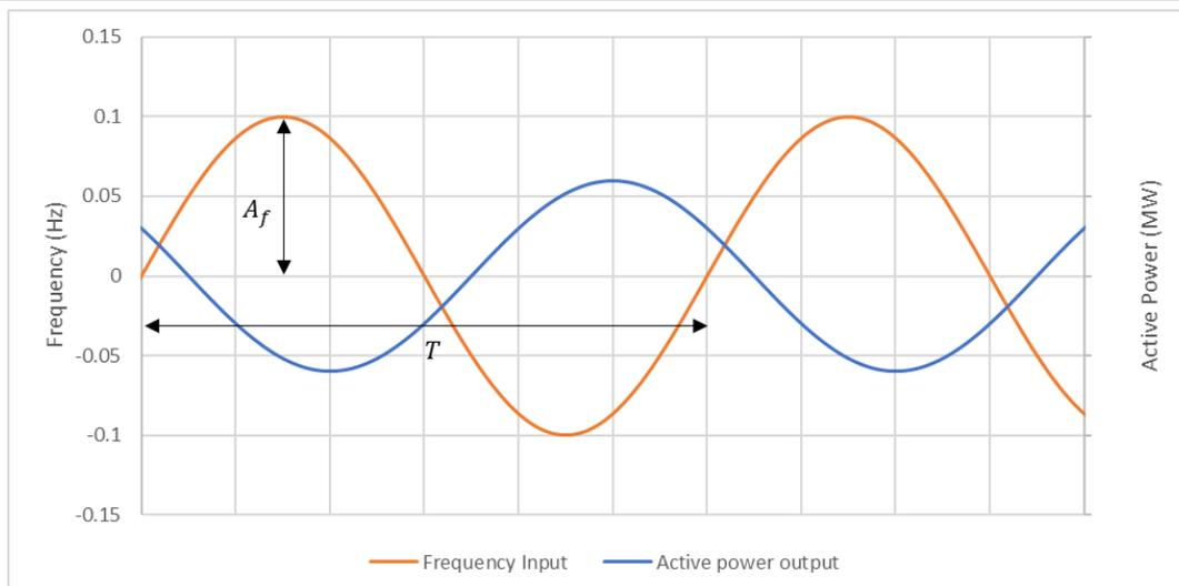
Figure 4. Input frequency signal for FCR-N sine tests
