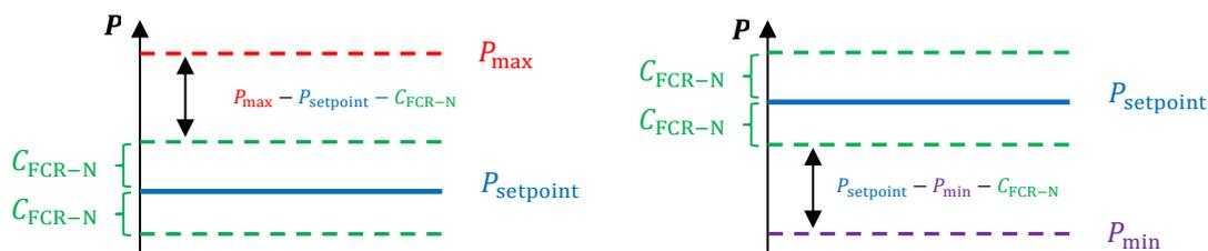
Figure 38: The limits of FCR-D capacity for a unit which is limited either by maximum active power or minimum active power while delivering FCR-N (FCR- D upwards in the left figure and FCR-D downwards in the right).
