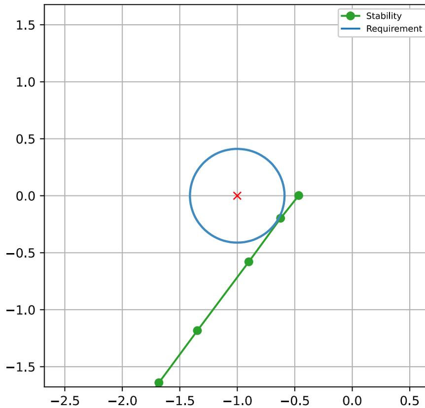
Figure 18. Example response of transfer function values (green dots) and transfer function (green line) of the open loop response which qualifies for the stability margin requirement (blue circle) and does not enclose the point (-1,0) (red cross).
