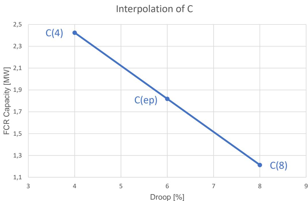
**Figure 34.** Third step of the linear interpolation to determine the actual capacity for droop levels between the minimum and maximum tested droop.
