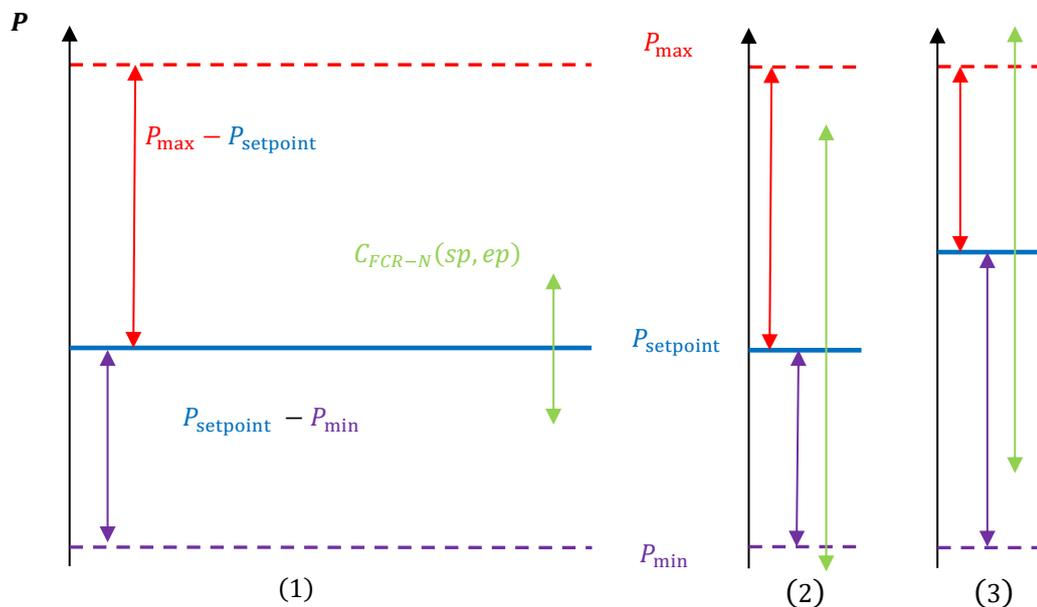
Figure 37: The three limits of FCR-N capacity for a unit which is limited either by prequalification test result (1), minimum active power (2) or maximum active power (3).
