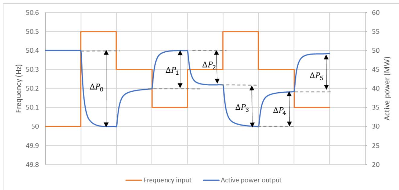
Figure 27. Example response (blue) from input frequency (orange) according to FCR-D Downwards step test
