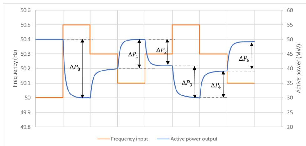
Figure 16. Example response (blue) from input frequency (orange) according to FCR-D Downwards step test.
