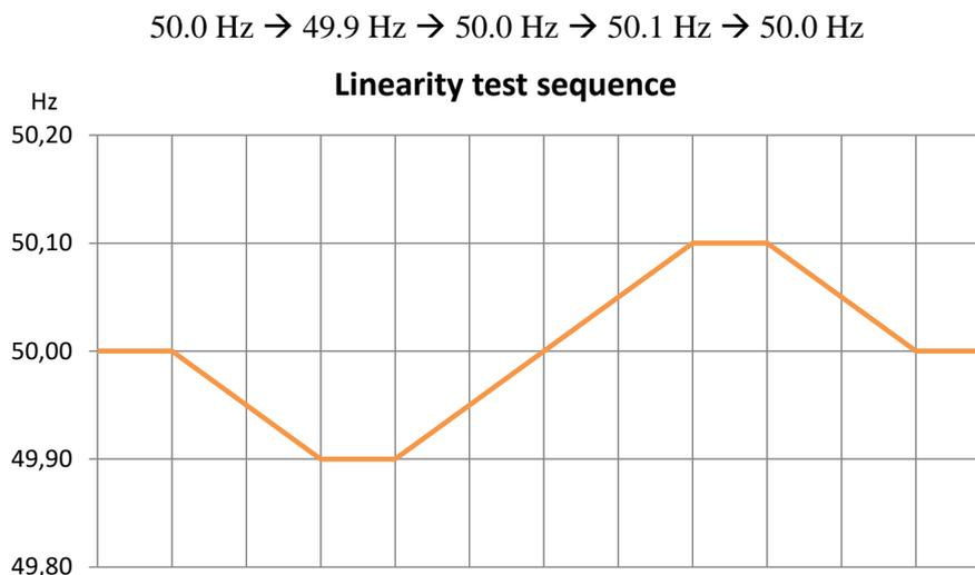
**Figure 11. FCR-N linearity test sequence to be performed for each setpoint and parameter set.**
