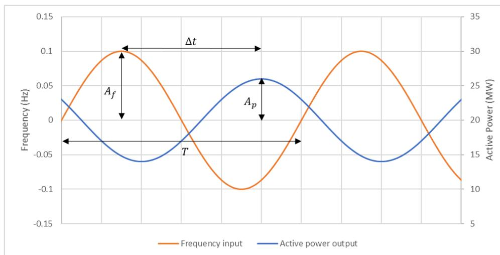
**Figure 17: Example response (blue) from input frequency (orange) for FCR sine test**
