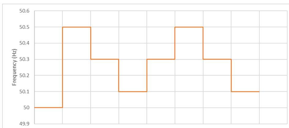
Figure 8. Input frequency signal for FCR-D Downwards step response tests
