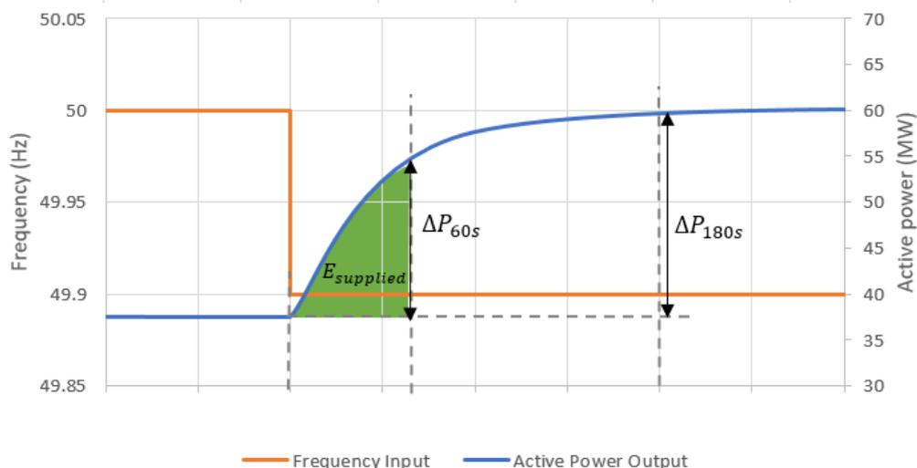
Figure 21. Example response of a single step, blue, from input frequency, orange, according to FCR-N step test from 50 to 49.9 Hz
