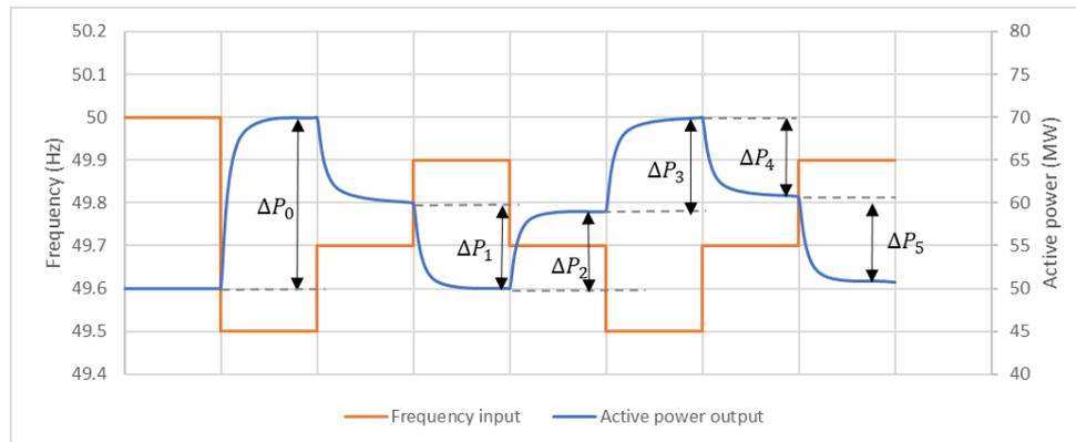
Figure 15. Example response (blue) from input frequency (orange) according to FCR-D Upwards step test.
