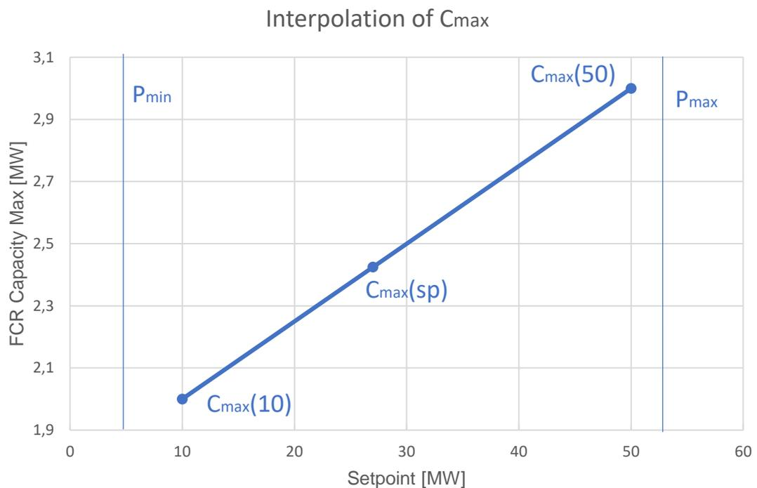
**Figure 32. First step of the linear interpolation to determine the maximal capacity for setpoints between the minimum and maximum tested setpoint.**
