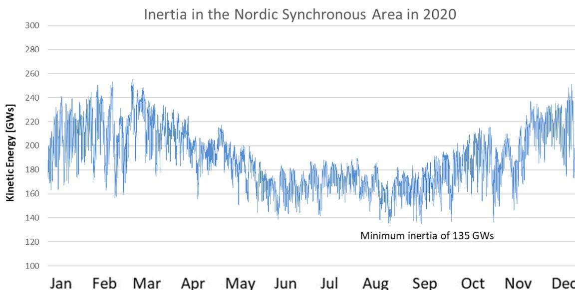
**Figure 3.** Estimated kinetic energy values (pre-disturbance values<sup>4</sup>) from the online kinetic energy estimation tool for the Nordic synchronous system in the year 2020.
