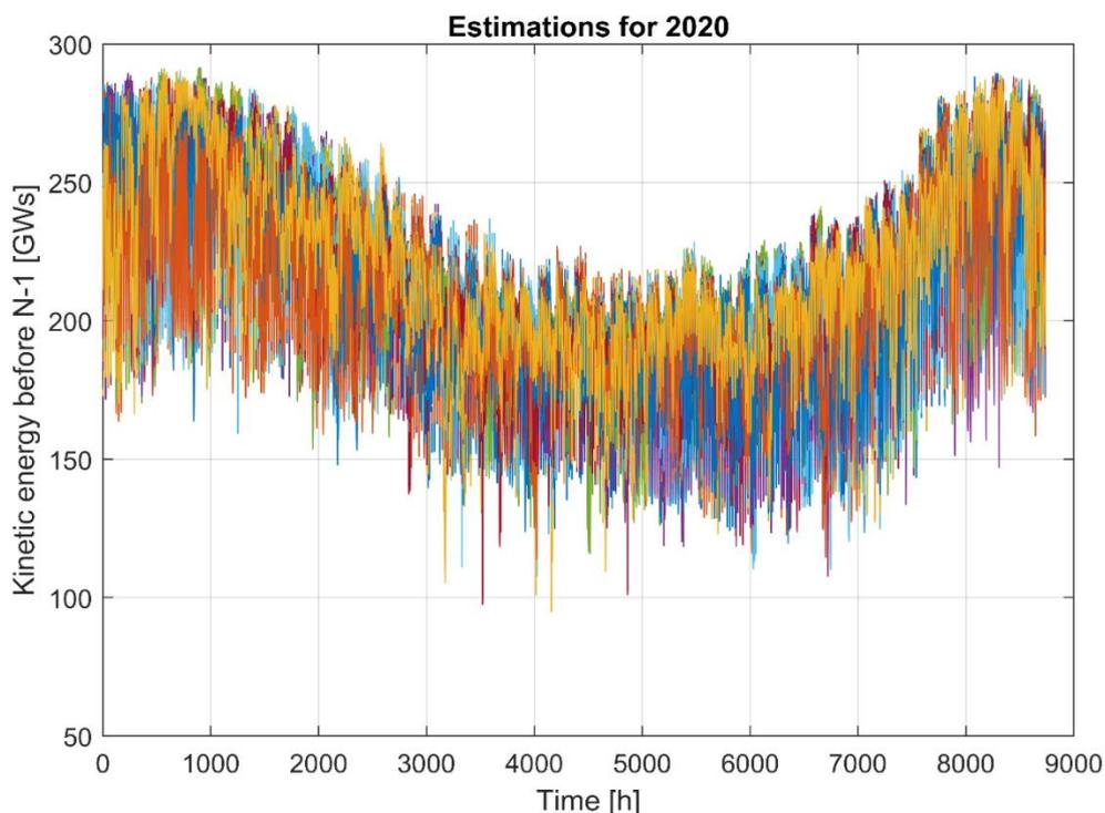
*Figure 5. The kinetic energy estimation for the base case of 2020 before the reference incident based on 31 input weather year data to the simulation model.*
