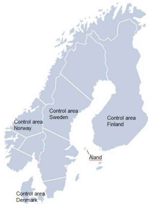
Figure 1: The interconnected Nordic power system and its control areas as defined in SOA. Note that only Eastern Denmark is part of the Nordic synchronous system.
