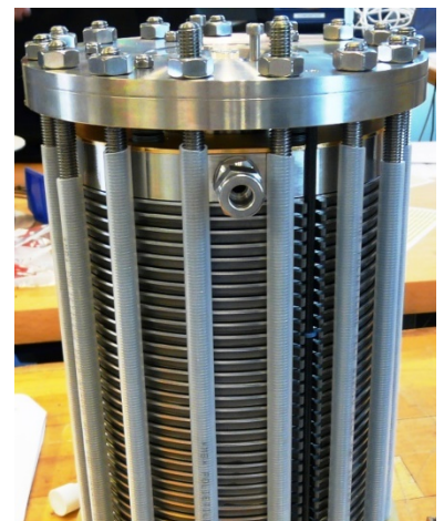
Figure 25. The IRD PEM stack with 33 cells.
