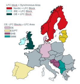
Figure 3. Currently applied European synchronous areas, LFC blocks and LFC areas. The LFC-block determination is not a term currently used in the existing Nordic configuration.
