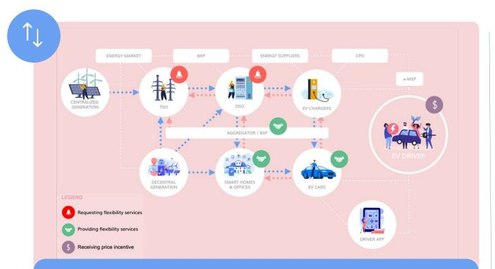
Energy from various nearby sources is locally stored, optimized, and supplied to the system via aggregators. By taking an active part in grid balancing and the larger energy transition, EV owners can gain from selling the excess electricity through an aggregator. As a participant in the market, the aggregator can help stabilize the electrical grid.
