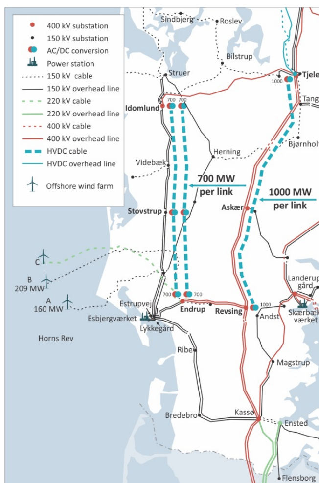
Figure 33: Layout of embedded HVDC multi-terminal link concept
