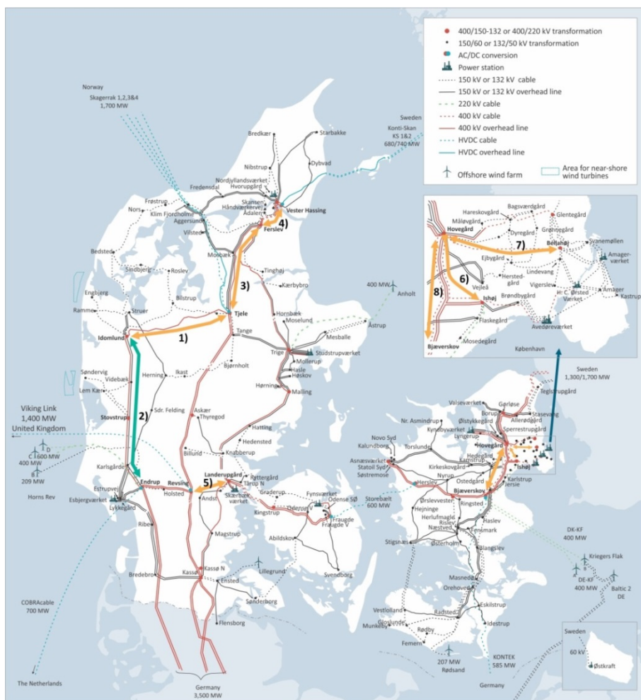
Figure 8 Required expansions of the 400 kV transmission grid (numbers indicate project IDs from the bulleted list on the previous page).
