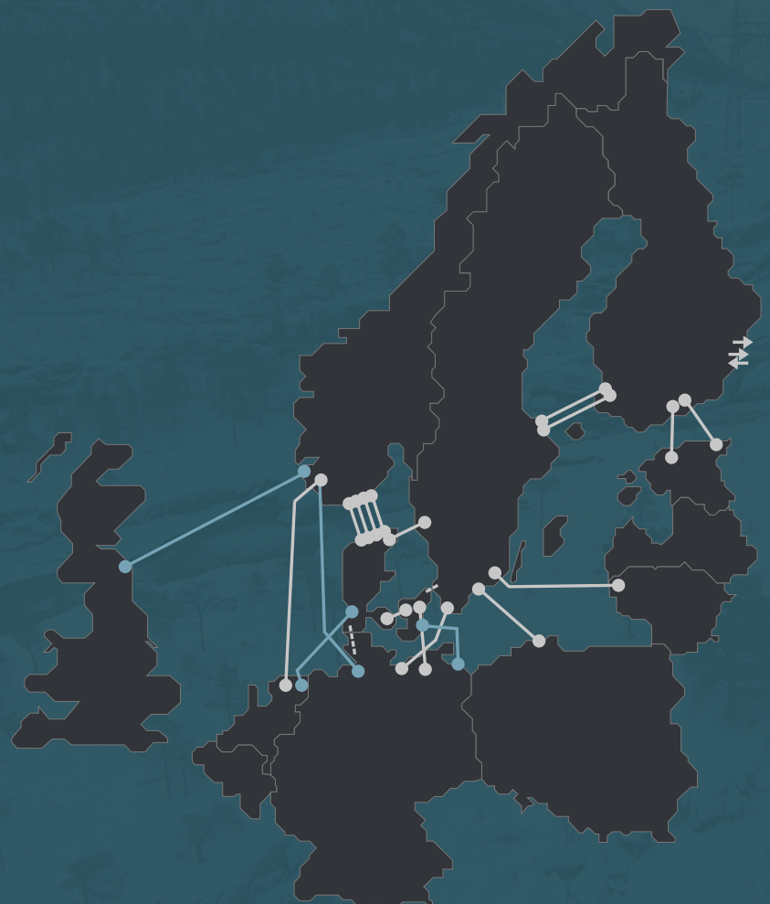
Figure 6 Overview of existing and planned HVDC interconnectors in the Nordic power system. Only those planned HVDC interconnectors with a final investment decision are included.
