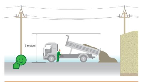
While the work is being performed, people, tools and other materials must not be located within the grey area, as marked in the illustration.
