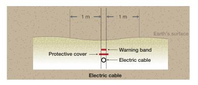
Remember drawings showing cable placement underground. If you strike a warning band or protective cover, then you are inside the safety clearance.
